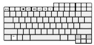
The computer uses hotkeys or key combinations to perform functions such as controlling the screen brightness and specifying where to display output.
