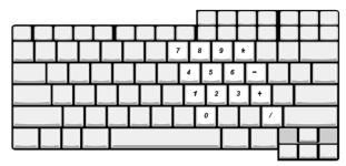
The embedded keypad functions like a desktop numeric keypad. It is indicated by small characters located on the lower edge of the keycaps. The embedded keypad can function in numeric mode or cursor-control mode.
