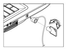
Wrap a computer security lock cable around an immovable object such as a table or locked drawer handle. Insert the lock into the notch and turn the key to secure the lock. Some keyless models are available.
